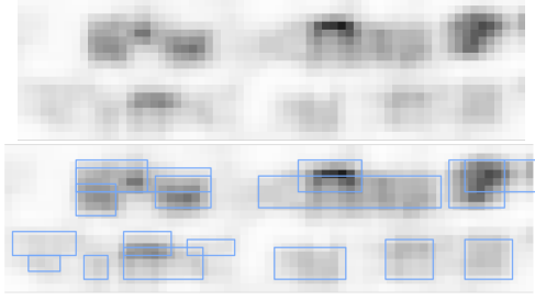
Figure 2. Close-up of tiretracks in SAR CCD image (left) with outline of each block (right)
