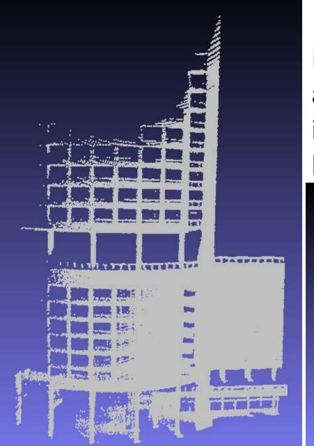
Missing points can also be caused by incomplete scan of building
