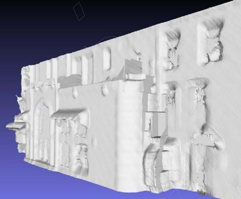
Mean depth of points below extrapolation area used to fit piece-wise linear approximation to missing façade.
