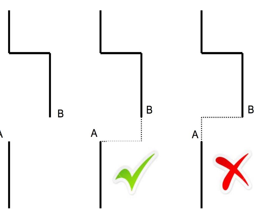
Gaps in the point-cloud are assumed to be caused by occlusions from the building architecture (e.g. window ledges, balconies).
